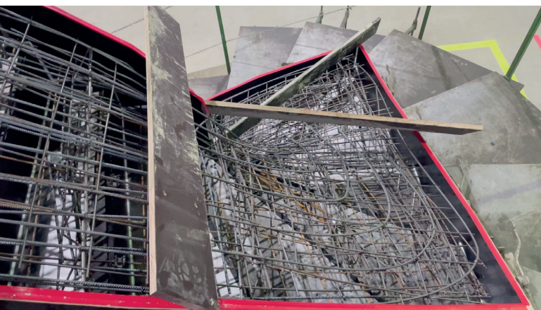
The use of steel fibres supports resource-efficient construction methods. On the left a staircase with conventional reinforcement, on the right a staircase with a combination reinforcement with the same performance characteristics.
