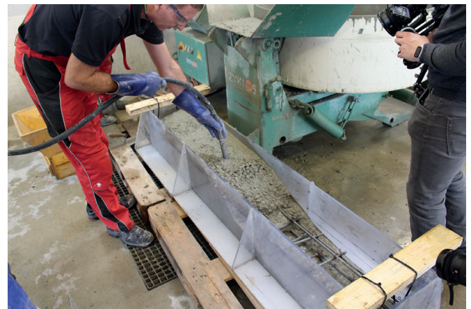
Extensive test program to determine the processability of the Stabils fibres in the Schwenk Technology Center of the company Schwenk Zement.
