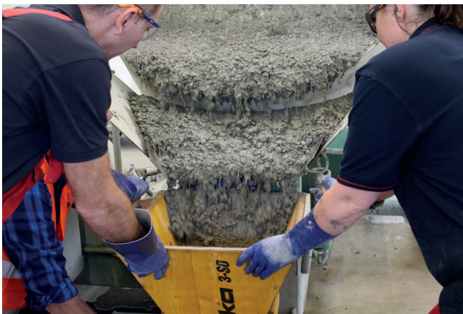
Extensive test program to determine the processability of the Stabils fibres in the Schwenk Technology Center of the company Schwenk Zement.
